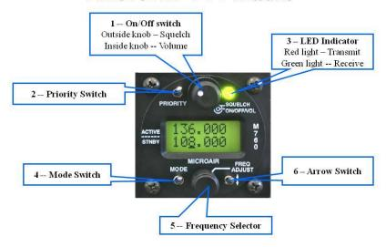
Figure 1 MicroAir Radio
