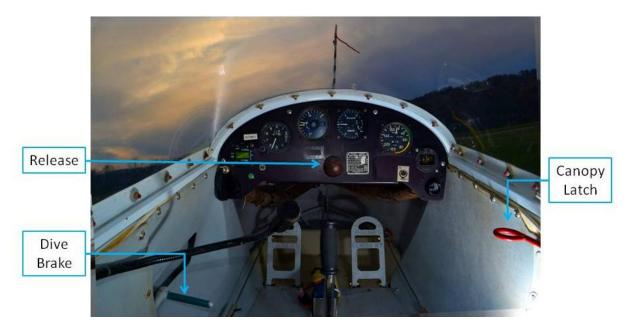
Figure 2 SGS 2-33A Front Cockpit
