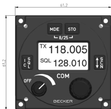
Figure 2-2 Mounting dimensions VHF transceiver
