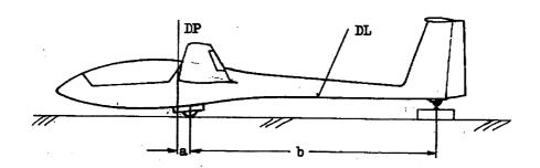
DATUM LINE (DL): under side of fuselage boom placed horizontal.
