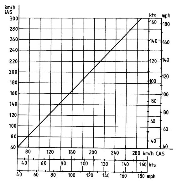
Fuselage nose pitot (without nose release) Pressure ports: Vertical tail fin pitot (with nose release) Forward fuselage side statics
